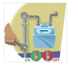
To isolate a ball valve, the handles needs to be turned in a clockwise direction so the arm is right angle to the rise piper.
